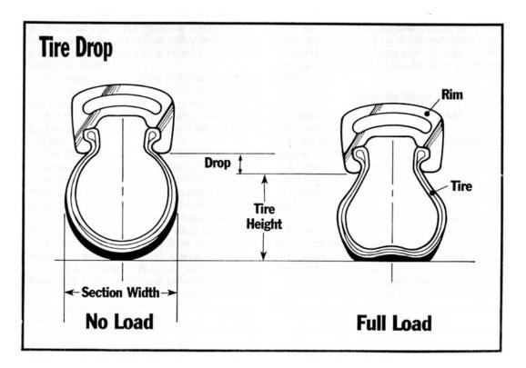
For example, suppose our typical 170-lb rider had two 30-lb bikes, one with 700x32C tires inflated to 100 psi and the other with 700x20C tires inflated to 100 psi. The load on each tire is 100 lb (simplifying things by assuming that each tire carries half the weight).
